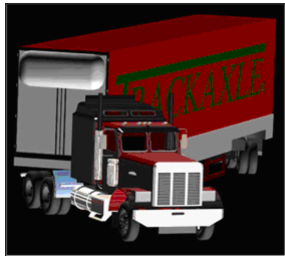
Computer rendering of a semi-trailer fitted with Trackaxle rear tyres. The rear tyres have turned so that they are facing the same direction as the prime mover’s tyres. Image used with permission from www.trackaxle.com.au .
